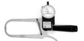
The Harpenden Skinfold Caliper is a precision instrument designed for use in the performance of skinfold thickness measurements (from which estimates of body fat are derived). The use of this instrument has been well established and documented over the past 40 years.
